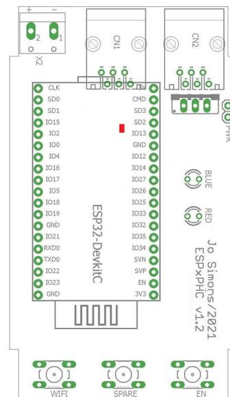
**Powering:** Fieldtests have shown that the module cannot be powered reliably from the PHC power supply as it draws upto 140mA of current, resulting in unpredictable behaviour. So therefore it is recommended to connect the ESP32-DevkitC to a USB power supply (or a spare PC) after removing the cap from the PWR connector on the PCB.
